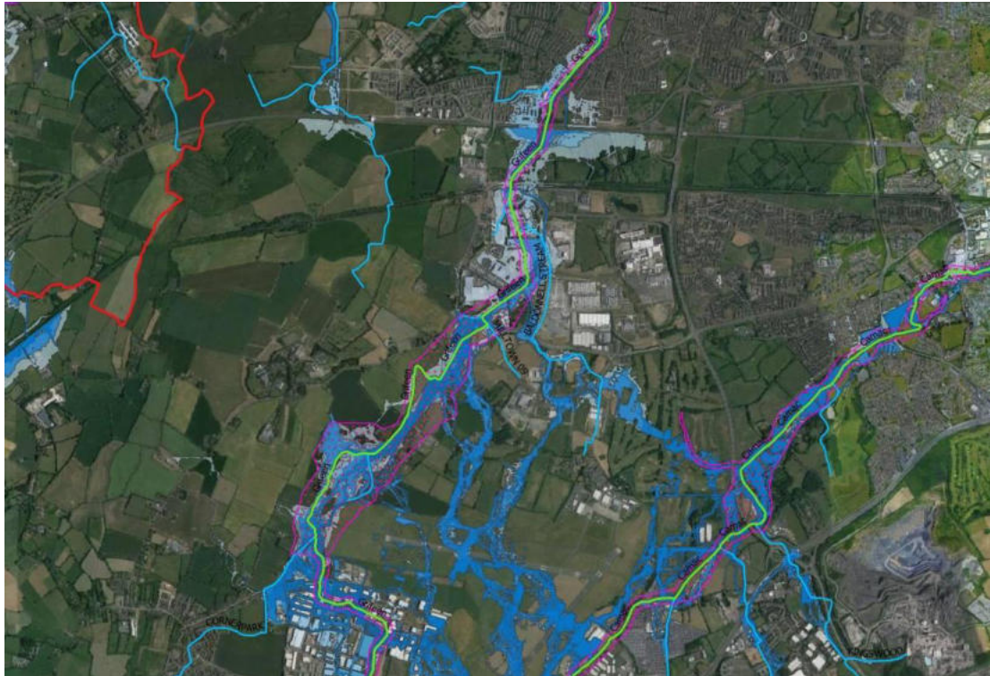
Figure 4.6 Indicated flood risk areas and Riparian Corridors (in pink) for Aungierstown – Ballybane
