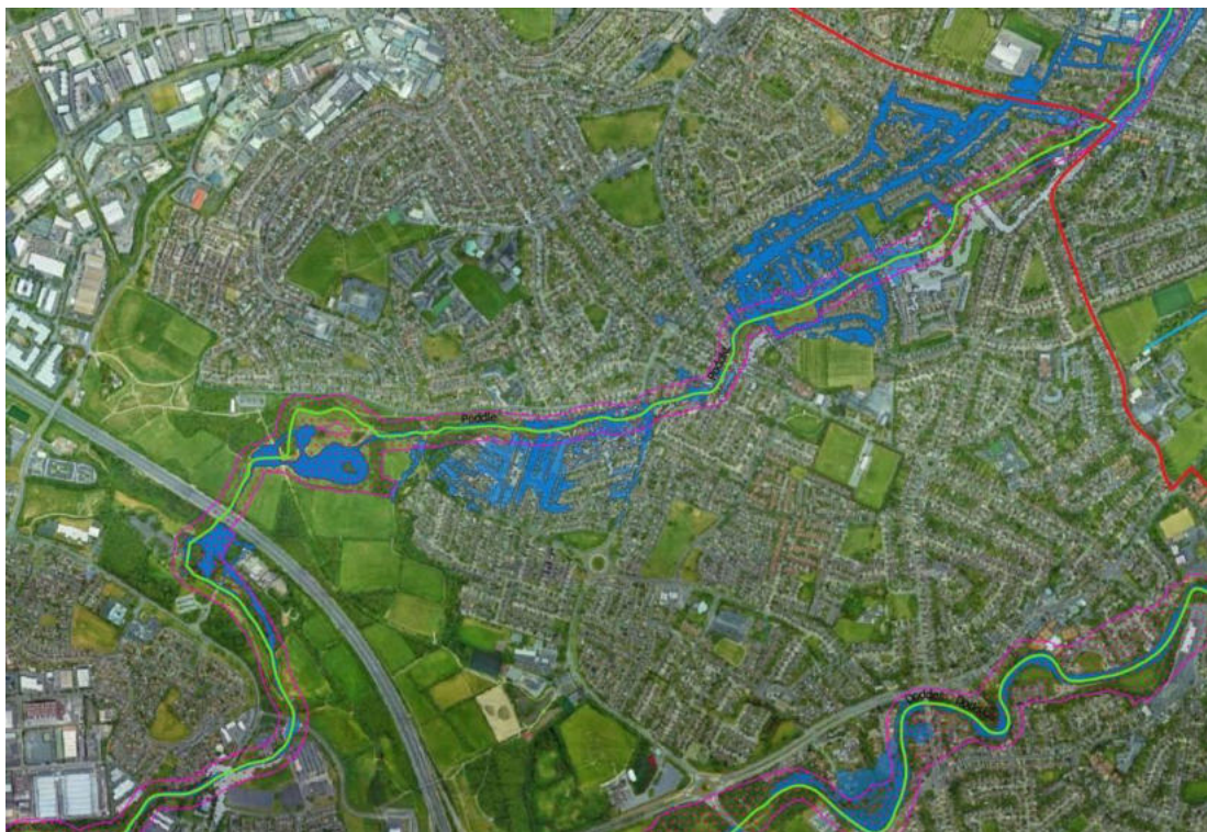
Figure 4.8 Indicated flood risk areas and Riparian Corridors (in pink) for Kimmage - Templeogue
